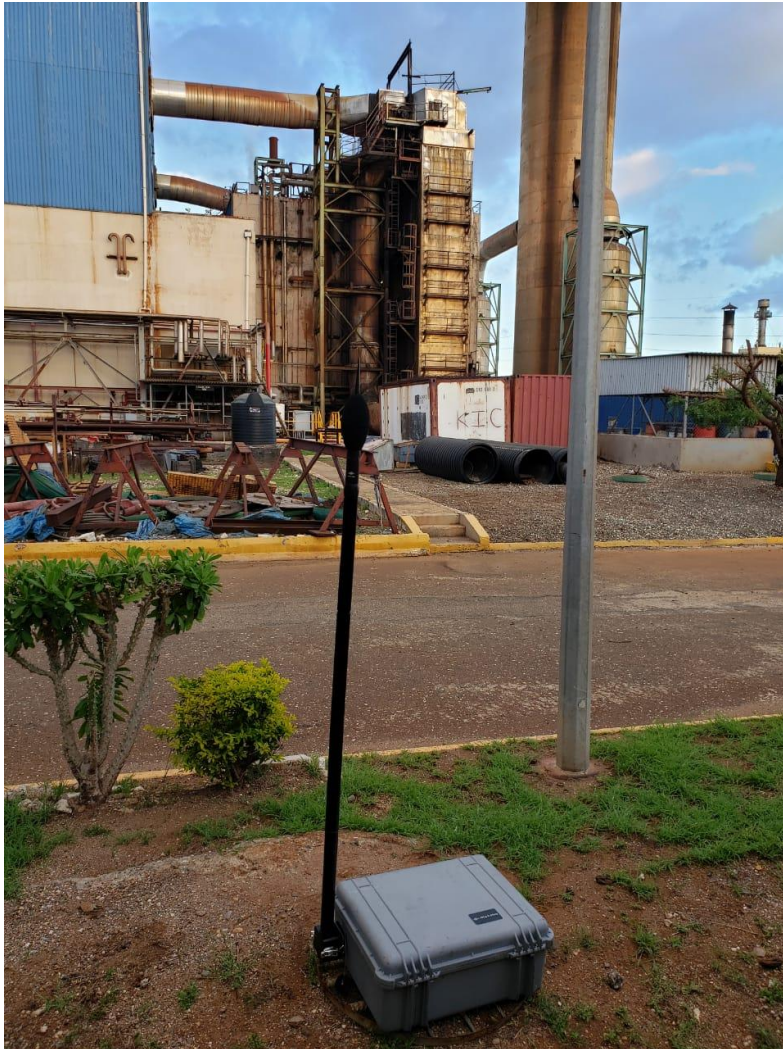
Plate 1 An example the Bruel and Kjaer outdoor noise kit setup on site, used for the 24-hour monitoring
