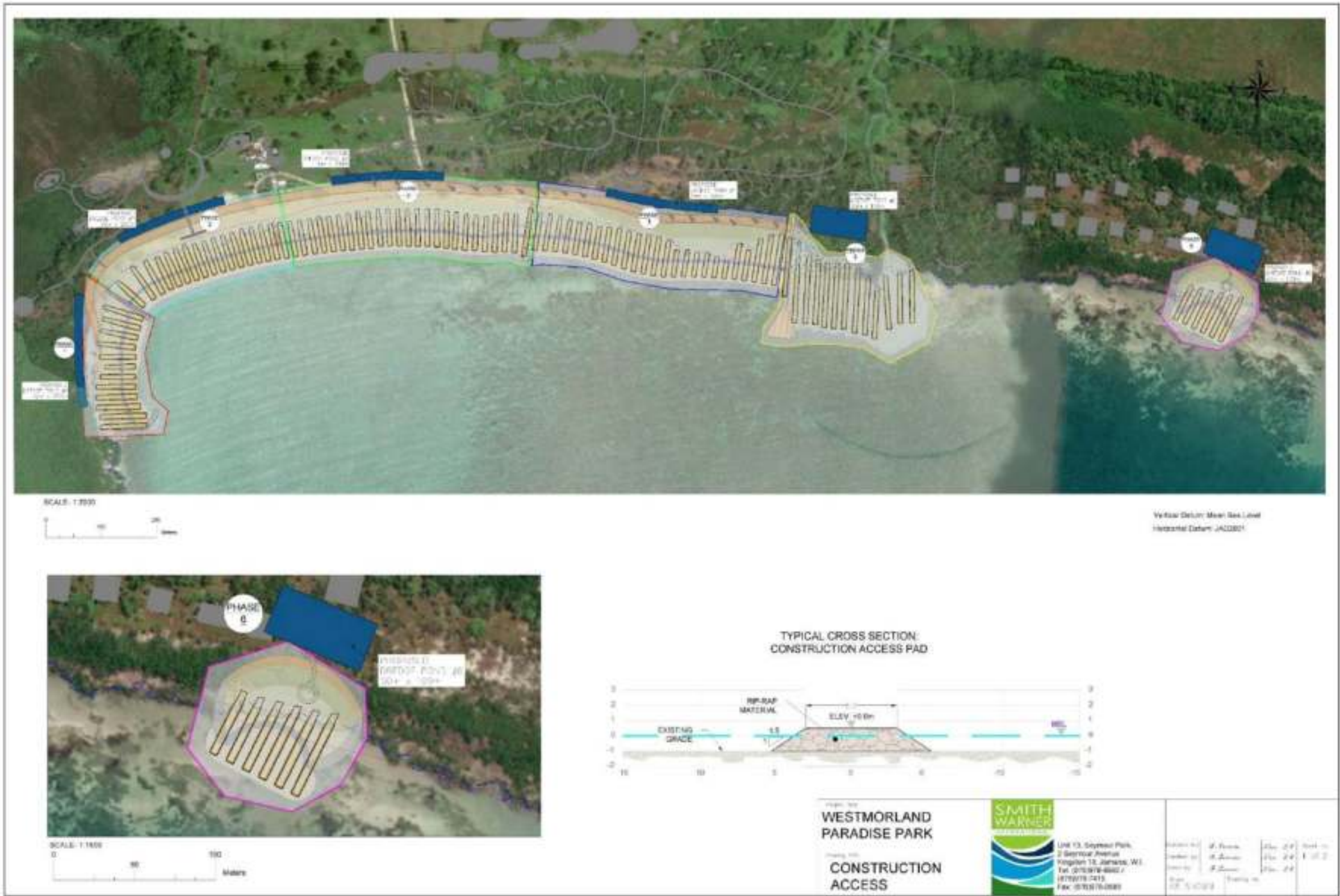
Figure 3-48 Phases, settling ponds and temporary access pad locations
