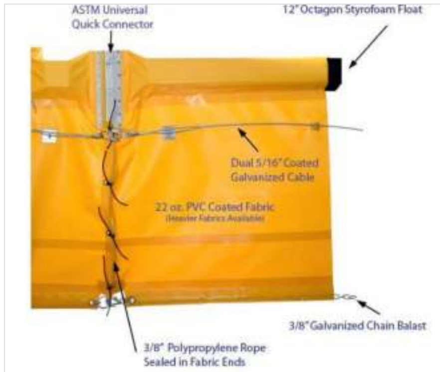
Figure 3-47 Specifications of a Mark III turbidity barrier
