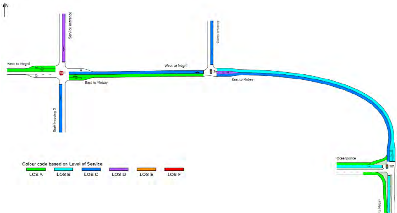
Figure 7-23 Level of service of hotel entrances with the implementation of the proposed solution – PM
