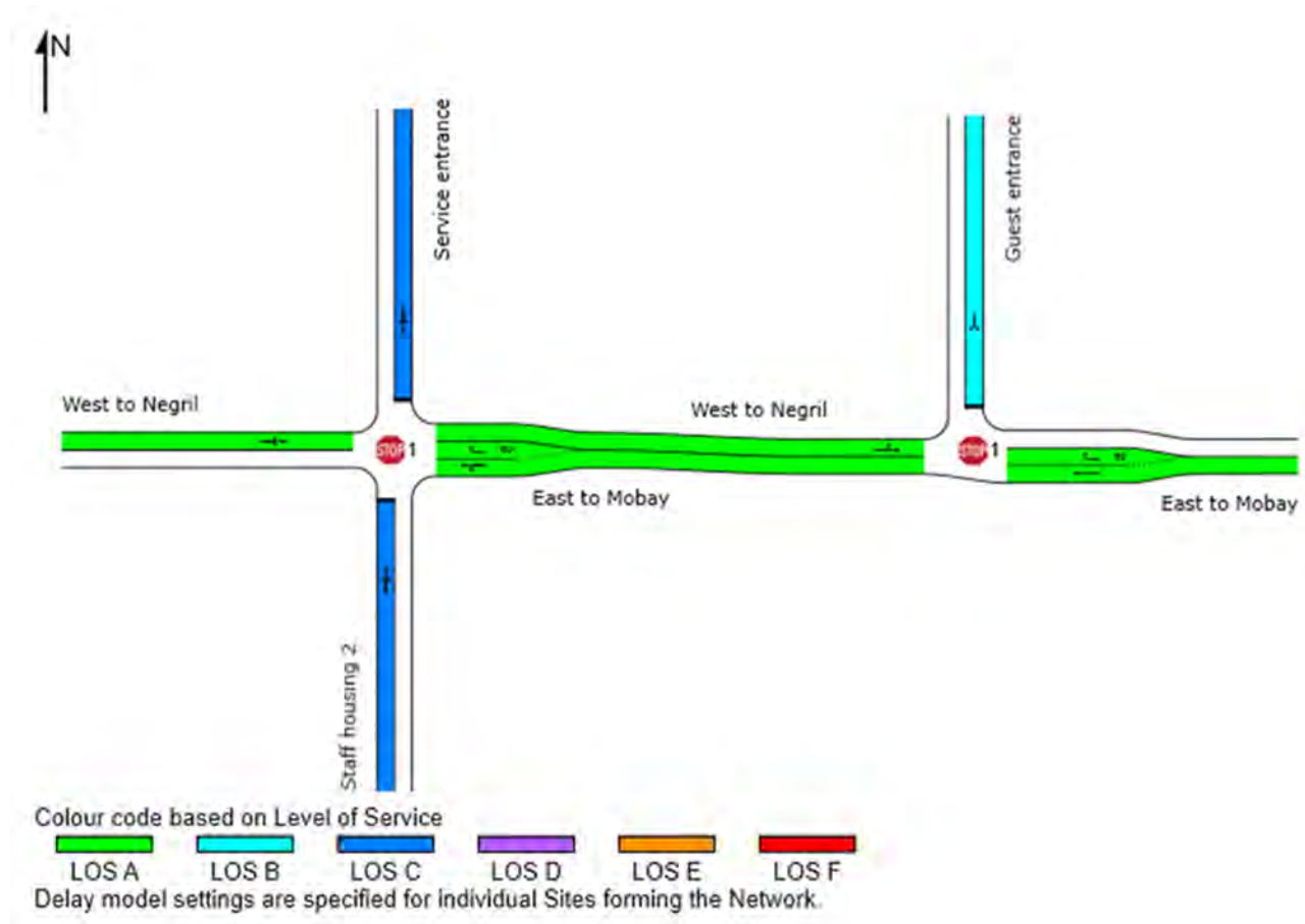
Figure 7-7 Level of Service during Pm peak during construction scenario
