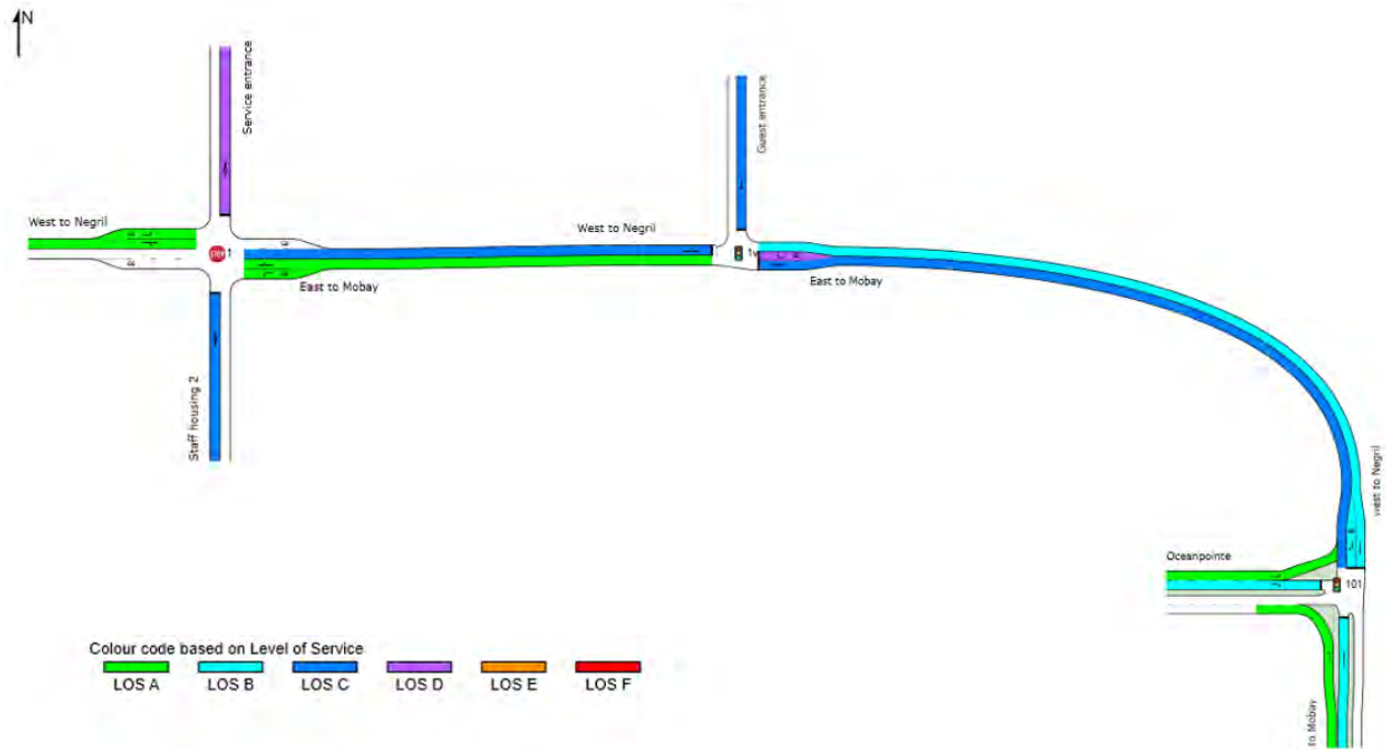
Figure 7-22 Level of service of hotel entrances with the implementation of the proposed solution - AM
