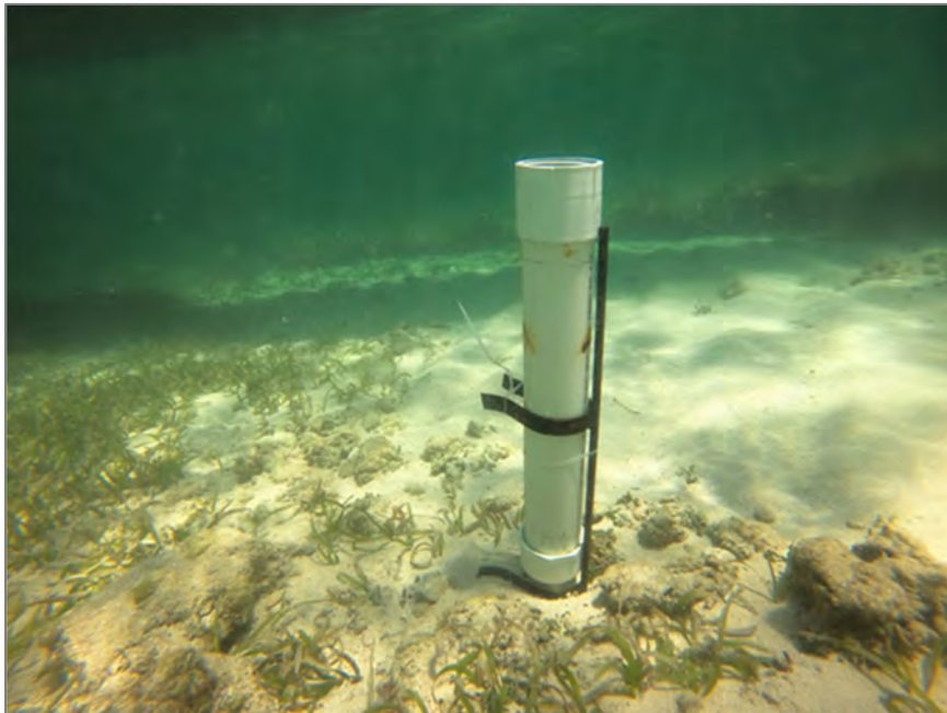
Plate 5-3 Example of sediment trap deployed
